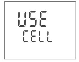
2 Press **<ENTER>** or **<CAL**\_\_> to confirm the selection of *USE CELL*.
