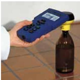
OxiTop® Control system uses software-controlled functions and infrared interface to communicate with the powerful OC 100 controller. This connection enables the simultaneous, group start, management, storage and tracking of 100 measuring heads, and tracks results on a large
