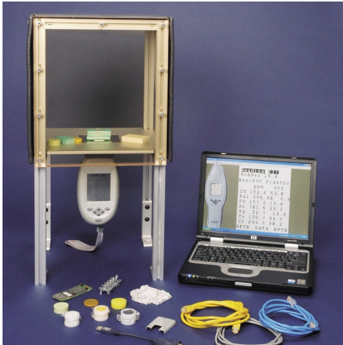
XLt 797 in benchtop test stand - remote operation via wireless PC link
